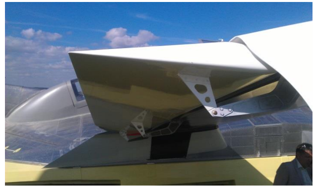
Figure 5. Airplane “Ivolga”. Aileron made using Aspro fabric 80 g/m 2 .
