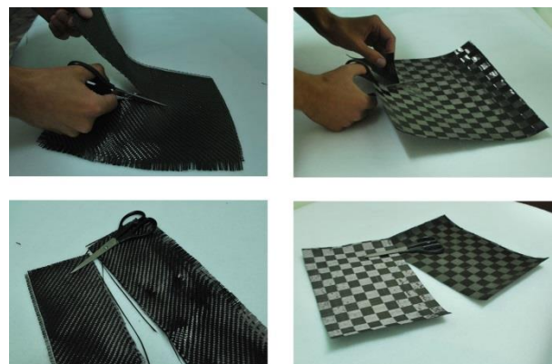
Figure 3. Ease of cutting and laying. Twill 3K 200 g/m 2 (left), Aspro fabric 24K 80 g/m 2 (right).
