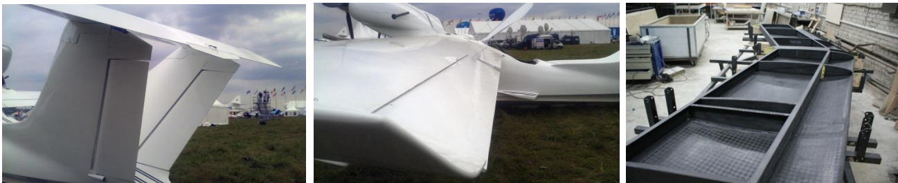
Figure 7. Ailerons, stabilizer, elevator and rudder aircraft L-42m made using Aspro fabrics 80 g/m 2 (left and center pic.). Stabilizer airplane “Ivolga” during assembly on the slipway (right pic.).
